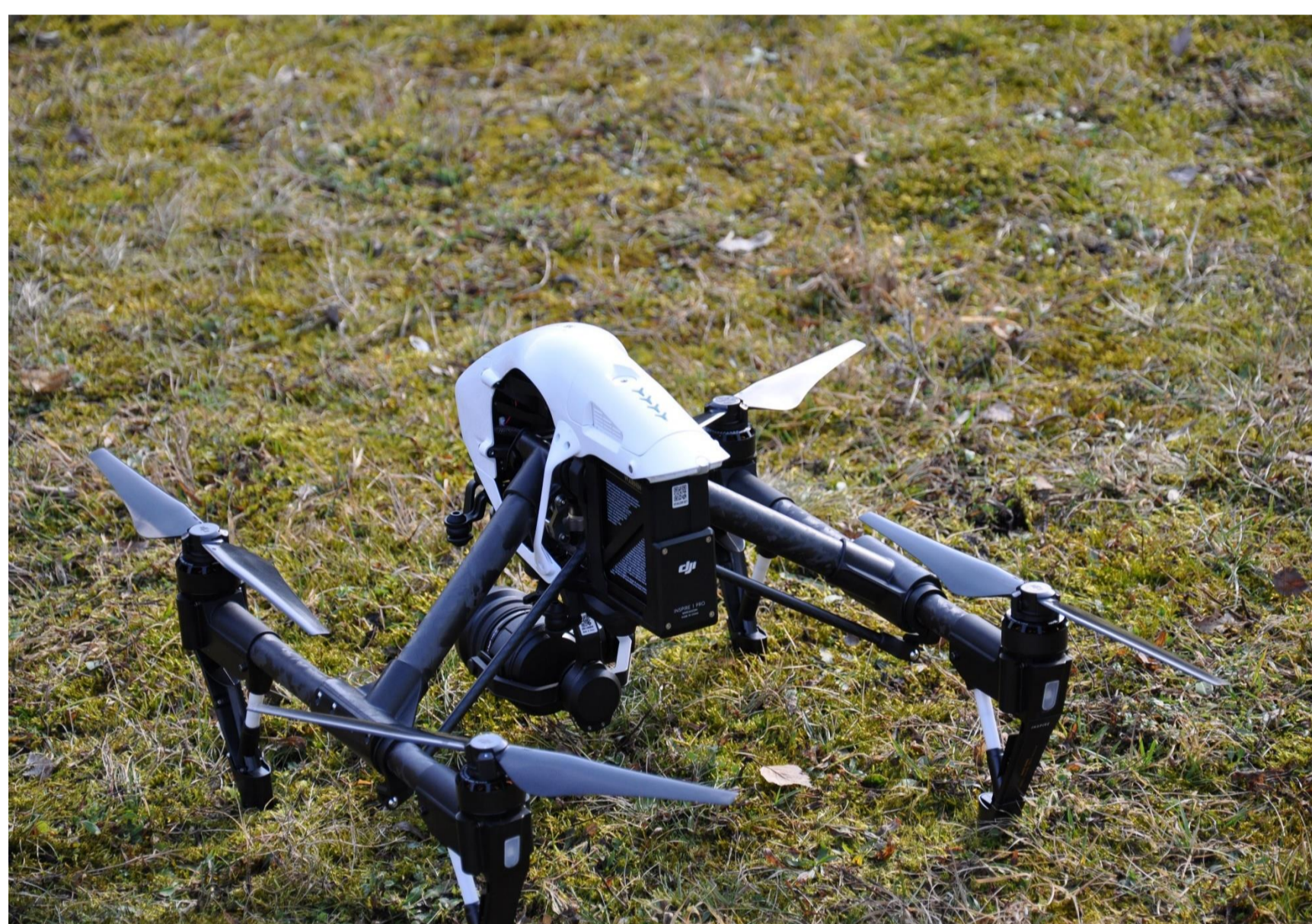
Fig. 2: DJI Inspire 1 PRO (X5) featuring a 16 MP on-board camera used for aerial photography
