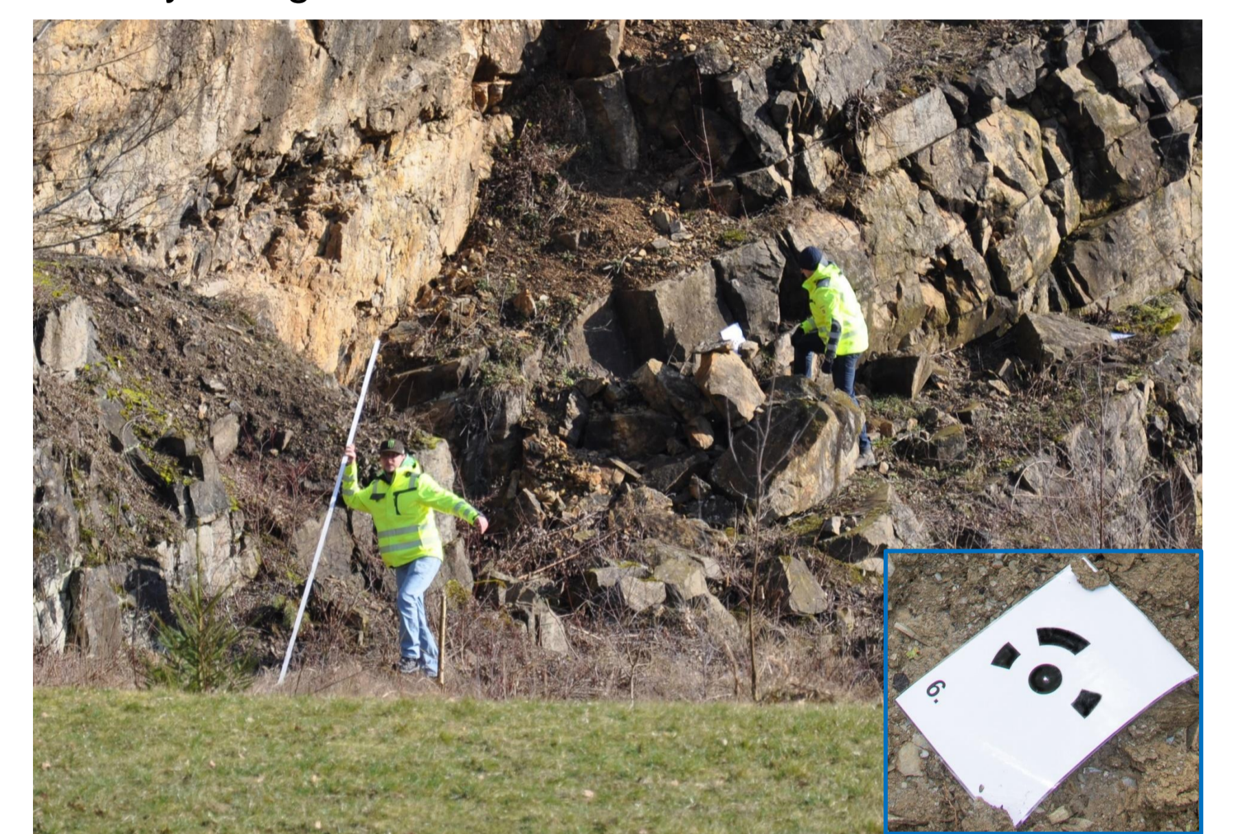
Fig. 3: Distribution and measuring of markers (blue box) in the area to georeference the final model (symbol on marker is recognized by photogrammetric software)
